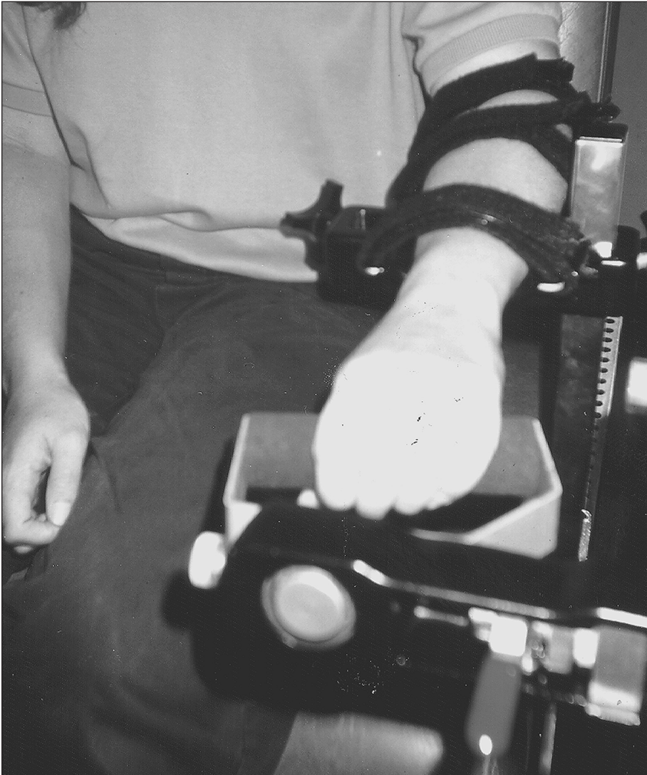
Isokenetic wrist extension strength measured with a lido dynamometer.
